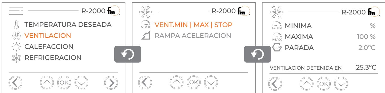
Accessing the ventilation menu, we configure the regulated ventilation output.
